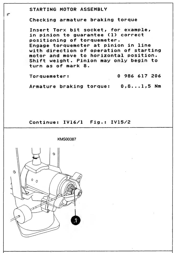
Checking armature braking torque
